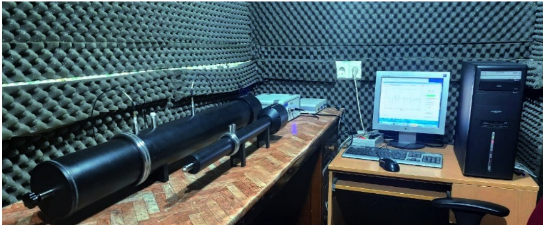
Fig. 1: Two-microphone impedance Tube setup
